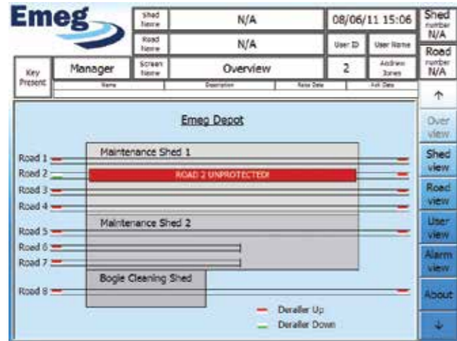
Typical screen image of main depot overview showing status of derailleurs.
